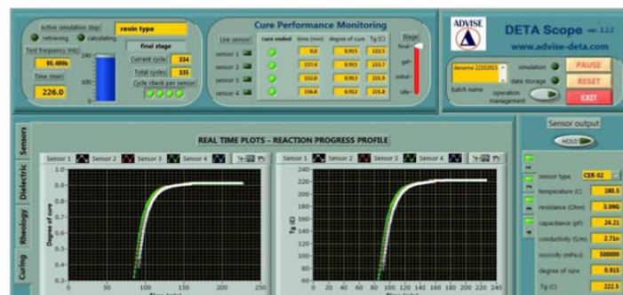
DETA SCOPE Cure Performance Monitoring tool showing the traces of degree of cure during a 4-sensor process
