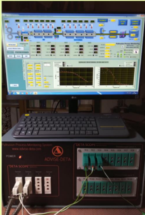
Cure Performance Monitoring System for industrial data acquisition from in-process sensors
