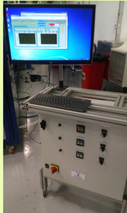
DETA-HEAT multi-zone thermal management system for self-heating tooling in composites processing
