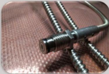
*Dielectric sensor for cure process monitoring*
